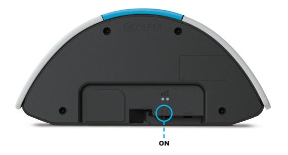
**6.** Set the ON/OFF switch to ON, 6 successive beeps indicates the start of the initialization.
