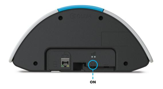
**7.** Set the ON/OFF switch to ON, 6 successive beeps indicates the start of the initialization.
